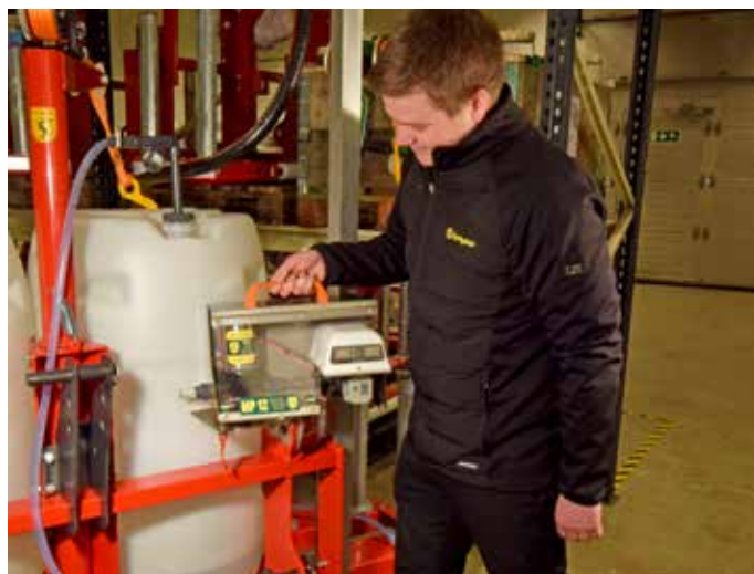
Figur 18 Demontert pumpe klar for lagring.
